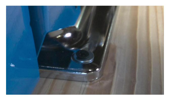
The mount is now complete. You may find it helpful on wooden baggers with sloped sides to place a long wood screw front and back to secure the vacuum to the frame. The mild slope has no impact on the effectiveness of the vacuum system.
