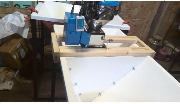
Place the small washers on the short wood screws and fix one through each corner of the lower mount of the vacuum system into the wood.
