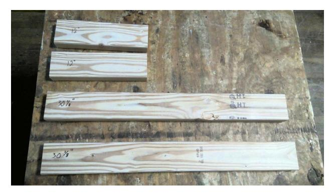
Lay the long boards out on the broad side and match with the short cuts set up on the short sides.
