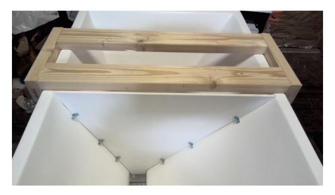
Place the vacuum system straddling the long boards aligned above the outlet of the hopper.
